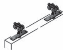
HANGER POSITIONED ON DOOR END WITH GUIDE ROLLERS ON OPPOSITE SIDES TO ALLOW DOORS TO STACK
